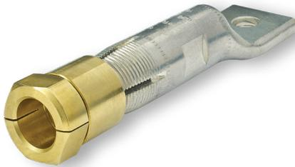
To achieve the connection, the nut is tightened with a standard wrench (open-end or adjustable). When tightened, the matching tapers evenly compress the copper body into the conductor, and the serrated inner surfaces bite for optimum pull-out strength. As the nut is tightened further, the hex portions snap off at their pre-set torque. The breaking torque is engineered into each size nut to a level that exceeds UL torque requirements.
